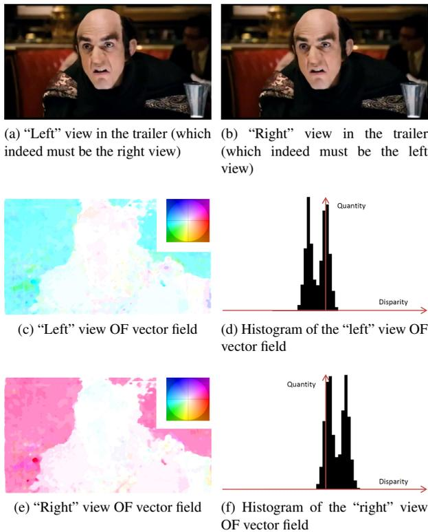
**Fig. 7:** Example of frame (a-b) with swapped channels detected by the proposed algorithm, corresponding OF fields (c, e) and OF vector histograms (d, f). Frame is taken from “The Smurfs” movie trailer. OF vector field is visualised using Middlebury color benchmark [1].
